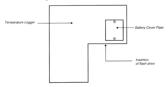
The Temperature Logger will be automatically energized when you plug your appliance into a 115V AC outlet.
